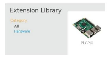
This will add GPIO blocks to the "More Blocks" category. Next you need to tell the Raspberry Pi to treat those particular pins as inputs. You can then replace the existing keyboard sensing blocks with the GPIO block, or add an "OR" operator as I have done in the example below.
