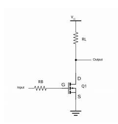
Here the MOSFET acts as a digital switch, which is turned on when the input is high and off when the input is low. The output is taken from above the MOSFET so when it is switched on then the output goes low and when the MOSFET is switched off then the output is pulled high through resistor RL. This means that the voltage shifter is inverting (you get the opposite at the output compared with the input). This is something we can handle in the software later.
