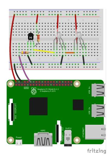
The MOSFET and LEDs need to be inserted the correct way around. In the case of the MOSFET then it should be inserted with the flat side facing towards the Raspberry Pi, in the case of the NeoPixel LEDs the two shorter legs are the ones on the left of the image. For the NeoPixels to fit then you may need to bend the two longer leads prior to inserting it into the breadboard.
