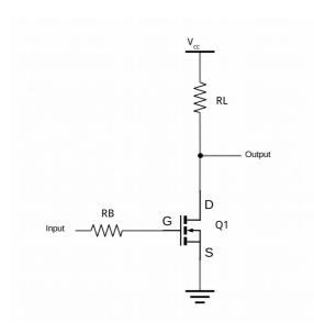
Here the MOSFET acts as a switch, which is turned on when the input is high and off when the input is low. The output is taken from above the MOSFET so when the MOSFET is switched on then the output goes low and when the MOSFET is switched off then the output is pulled high through resistor RL. This means that the voltage shifter is inverting (you get the opposite to the output compared with the input). This is something we can handle in the software.
