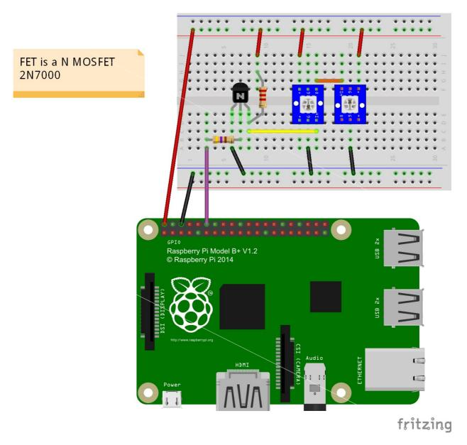
Note that the two NeoPixels are mounted the opposite way around from each other. This is so that the output from the first is close to the input for the second NeoPixel.
