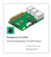
This will add Raspberry Pi GPIO blocks below the "My Blocks" category. These include the ability read the state of the GPIO ports (used with switches) or set the output of GPIO ports (used with the LED later).
